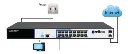
**Step 2.** Manually changed the computer IP address to 192.248.254.X (X is 2  $\sim$  254), subnet mask is 255.255.255.0
