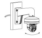
3 Screw up and complete the fixation of adaptor
