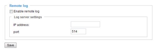
You can configure the video server to send the system log file to a remote server as a log backup. Before utilizing this feature, it is suggested that the user install a log-recording tool to receive system log messages from the video server. An example is Kiwi Syslog Daemon. Visit http://www.kiwisyslog.com/kiwi-syslog-daemon-overview/.
