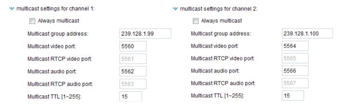
Unicast video transmission delivers a stream through point-to-point transmission; multicast, on the other hand, sends a stream to the multicast group address and allows multiple clients to acquire the stream at the same time by requesting a copy from the multicast group address. Therefore, enabling multicast can effectively save Internet bandwith.
