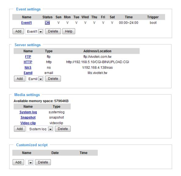
When the Event Status is **ON**, once an event is triggered by motion detection, the video server will automatically send snapshots via e-mail.
