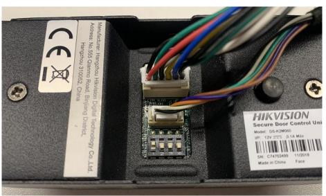
2) If you need to replace the second door lock interface, turn the NO.2 digit on
