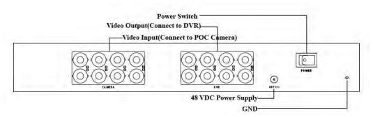
NOTE DS-1TP04I provides 4-ch video inputs and outputs.
