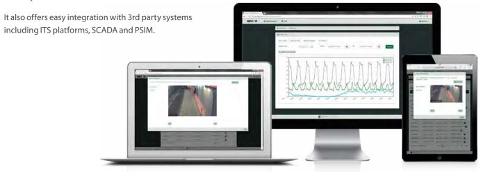
In complex architectures Traffic Hub can work as a proxy server forwarding all the events collected from the cameras to 3rd party software or VMS platforms. This features definitely simplifies the integration process avoiding the communication with every single camera connected on the network. The same communication interface enables 3rd party applications to disable some or all the detection features in the case of road maintenance.
